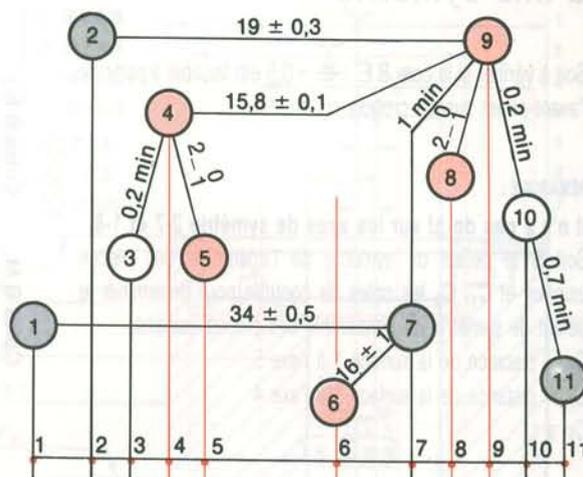
$$\begin{aligned} \text{Cf}_{9-3} \text{ moy} &= \text{C B.E.}_{9-4} \text{ moy} + \text{C B.E.}_{4-3} \text{ moy} \\ &= 15,8 + 0,425 = 16,225. \end{aligned}$$
